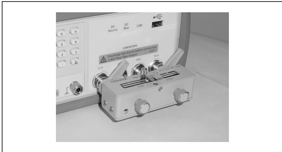
Figure 7-19 Connecting a shorting bar
